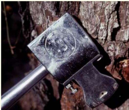
A Hypohatchet delivers a set amount of herbicide into a tree on impact. It has a hollow handle attached by flexible tubing to a bottle containing the herbicide.
