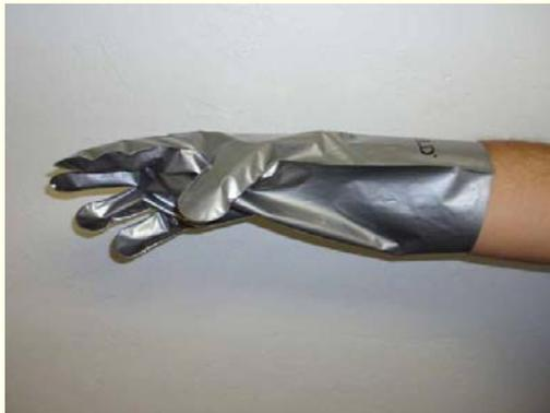
**Barrier Laminate:** a multi-layer, laminated, foil-like plastic film used to make gloves or aprons worn to protect the skin from contact with harmful chemicals.
