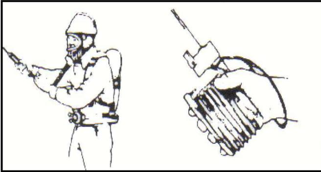
**Direct reading detection device:** An air-sampling device used to measure the concentration of a toxic gas in the air at a fumigation site.
