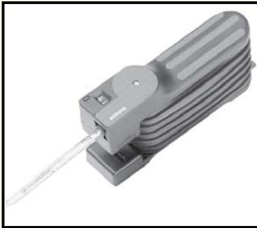
Dräger colorimetric tube and pump gas collector
