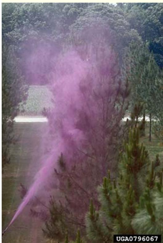
**Spray distribution research using a high-pressure, single-nozzle ground sprayer (no drift suppressants).** Photo courtesy L.R. Barber, USDA Forest Service, Bugwood.org
