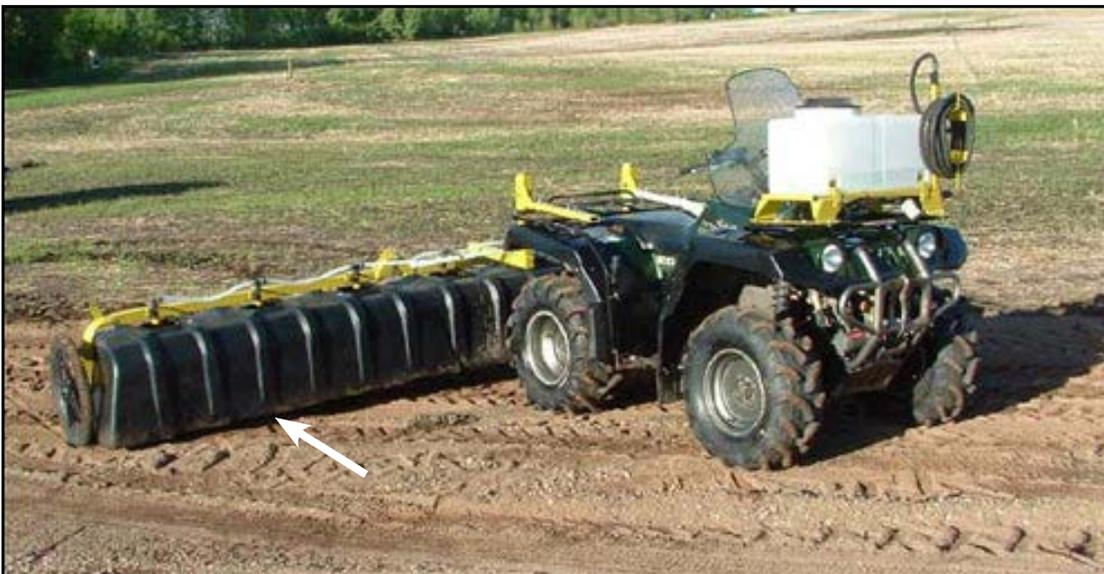
**Fig. 6. Boom sprayer with a fabric curtain (arrow) to help protect the applicator from spray drift.** Photo Agshield Co., Ltd.
