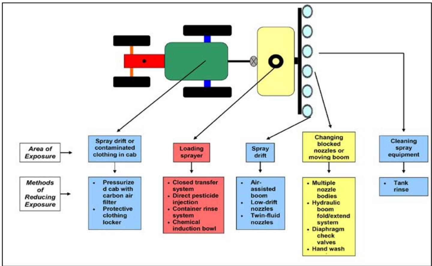
Fig. 2. Areas of potential pesticide exposure and engineering controls to reduce exposure. From "Solutions for Safer Spraying," Cornell
