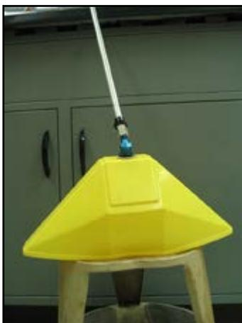
**Fig. 7. A plastic shield for a single-nozzle spray wand.**
