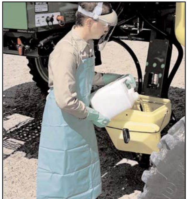
Fig. 4. Handler adding pesticide concentrate to an induction bowl. Cornell Cooperative Extension Svc.
