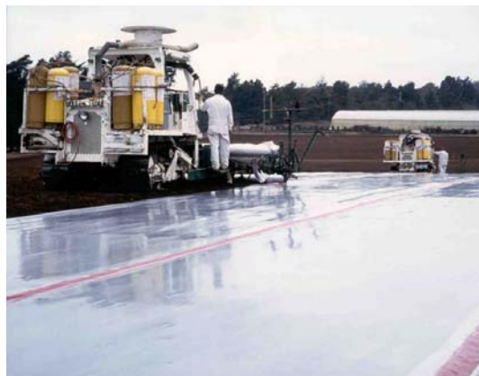
Soil injection of methyl bromide and chloropicrin followed by immediate tarping
